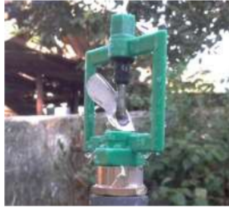
Figure 1. Butterfly rotary sprinkler
